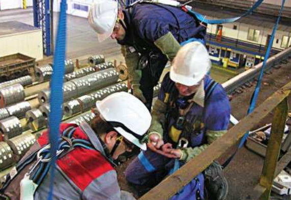
Tenzometrické meranie žeriavovej dráhy v U.S.Steel / Tensometric measurement of the crane track in the U.S.Steel company // Tensometrische Messung der Kranbahn in U.S.Steel
