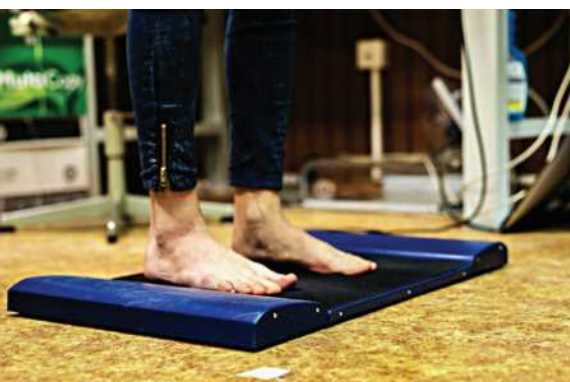
Tenzometrická plošina podobarometra MS Postural / Tensometric platform of MS Postural podobarometer // Tensometrische Plattform des Baropodometers MS Postural
